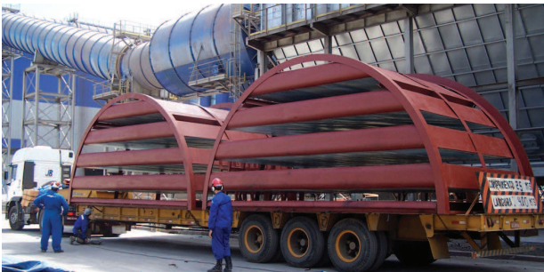
Stack Silencer for South American Power Plant
