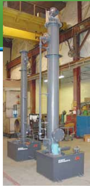
Landfill Gas and Biogas Scrubbing: PVC constructed Packed Bed Scrubbers for hydrogen sulfide ( H_2S ) removal from methane ( CH_4 ) gas
