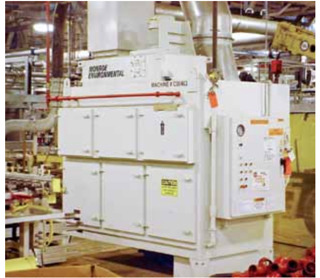
8,000 CFM Oil Mist Collector to filter parts washer exhaust at an automotive manufacturing facility
