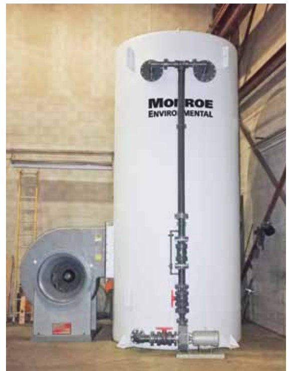
20,000 CFM Packed Tower Scrubber, FRP construction to remove acid and alkaline fumes from casting processes
