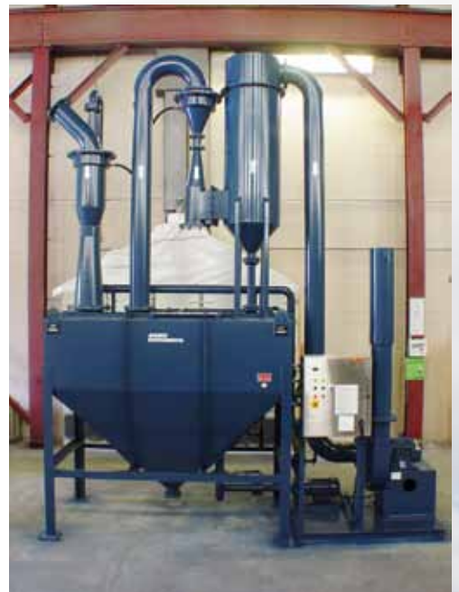
1,000 CFM Scrubbing System to remove lime dust from a chemical manufacturing process. (From left): Ejector Venturi, liquid clarification tank, high energy Venturi Scrubber, and cyclonic separator. The unit was designed to achieve 95% efficiency on 0.5 micron particles.
