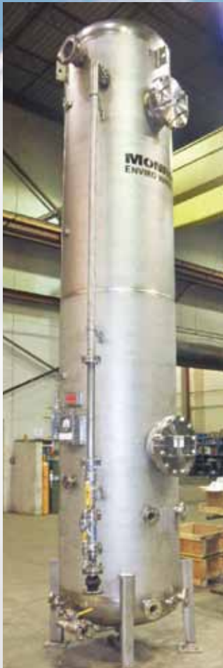
1,500 CFM Packed Tower Scrubber, stainless steel pressure vessel construction to remove H 2 S from syngas for a diesel fuel conversion process
