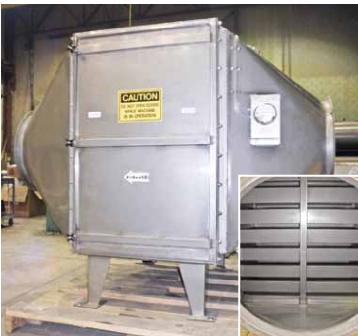
8,000 CFM Carbon Tray Adsorber for a recycling facility, shop assembled with stainless steel housing and differential pressure gauge
