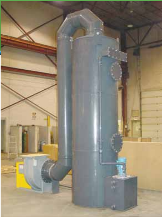
3,500 CFM Packed Tower Scrubber, PVC construction for HCl removal
