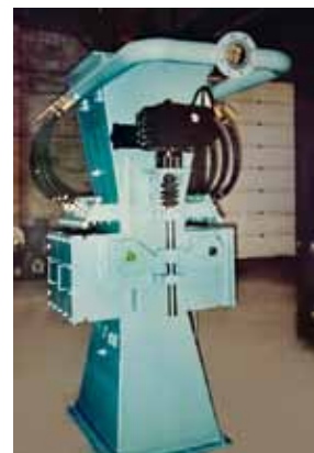
Adjustable, rectangular Venturi Scrubber throats for wet dust collection
