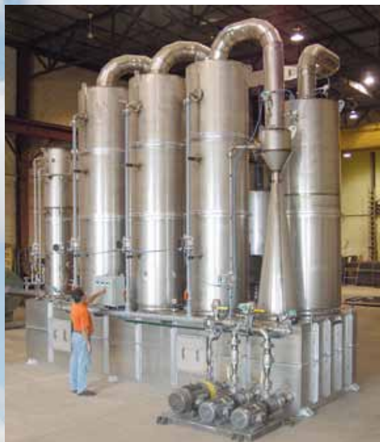
Stainless steel Multi-Stage Scrubbing System to treat exhaust from a toxic gas incineration process
