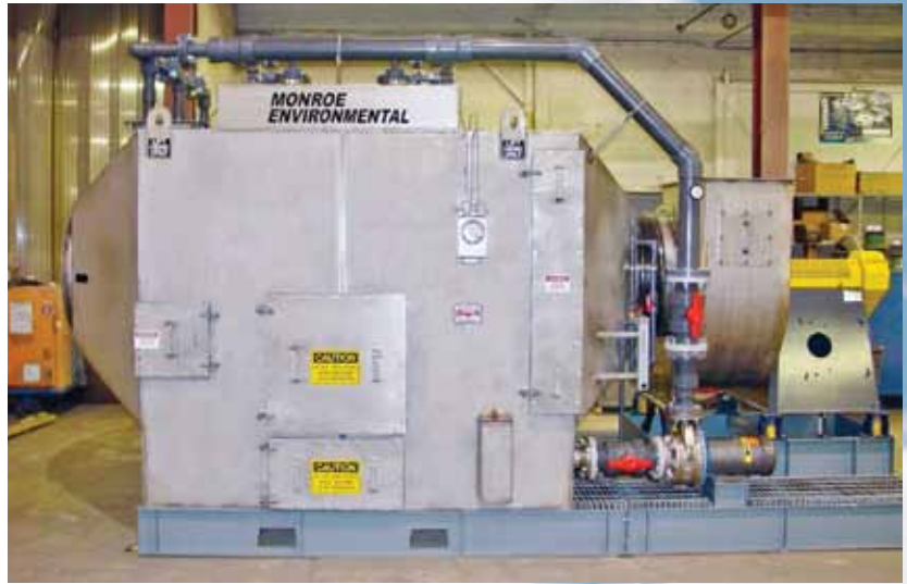
13,500 CFM skid-mounted Horizontal Packed Bed Scrubber, stainless steel construction to scrub acid and caustic fumes
