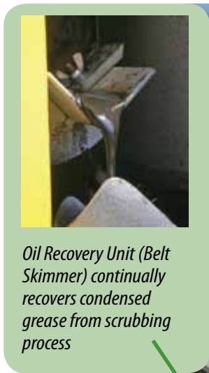
15,000 CFM Scrubbing System to condense and reclaim vaporized grease and remove hydrocarbon fumes from a chemical manufacturing process. The system includes a Dual Throat Venturi Scrubber with drag conveyor, Oil Recovery Unit, and Packed Bed Scrubber for odor control.
