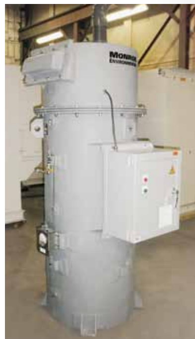
200 CFM Carbon Adsorber, FRP construction, with control panel for H 2 S removal at a municipal lift station
