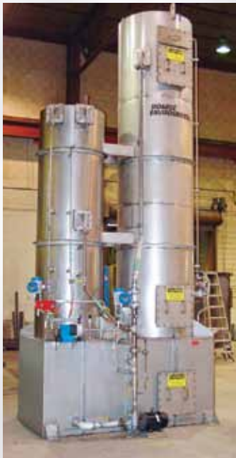
3,500 ACFM High temperature scrubbing system, stainless steel construction with inlet quench and vertical packed bed for SO 2 removal from RTO exhaust
