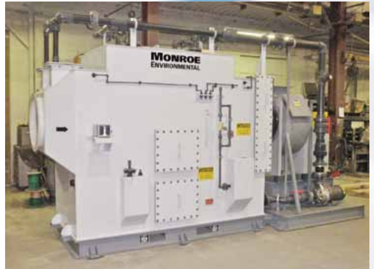
Kiln, RTO, and Incinerator Scrubbing: 7,500 CFM skid-mounted Horizontal Packed Bed Scrubber, polypropylene construction to capture and remove NaOH fumes from kiln exhaust
