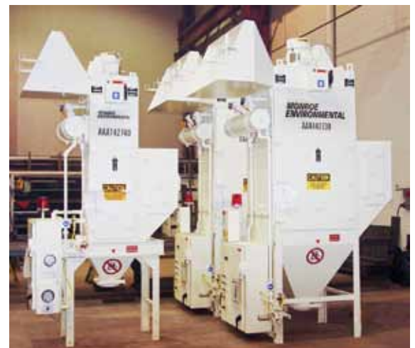
(1) 500 CFM and (2) 1,500 CFM Cartridge Dust Collectors for welding and wire brush deburring at an automotive plant
