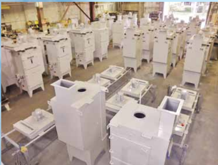
Assembly of 37 Spiral Tube Oil Mist Collectors for an automotive engine and transmission machining operation
