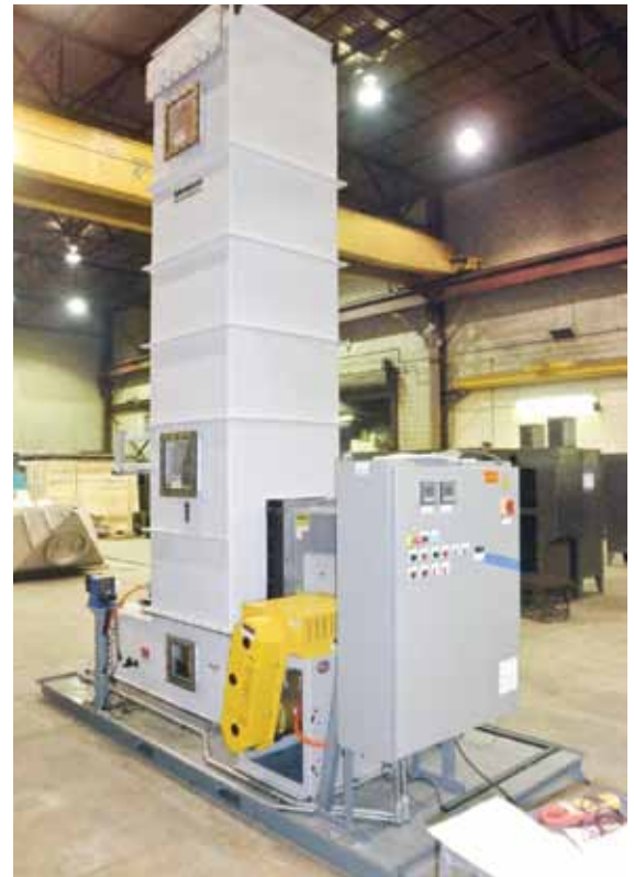
5,000 CFM Packed Tower Scrubber, polypropylene construction to remove acid gases from chemical tanks at a recycling facility
