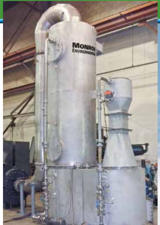
6,000 ACFM Two-Stage Scrubbing System, stainless steel construction with adjustable Venturi followed by Packed Bed Scrubber to treat exhaust from a flame lamination process
