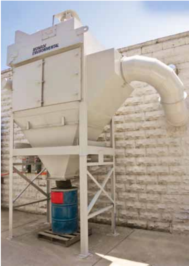
6,000 CFM Cartridge Dust Collector with inlet duct and storage drum exhausting a sandblasting and paint spraying operation
