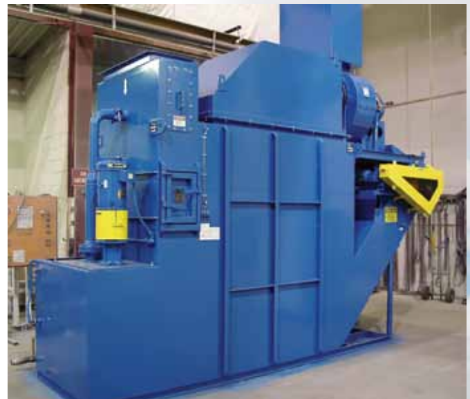
9,600 CFM Dual Throat Venturi Scrubber for boiler exhaust scrubbing
