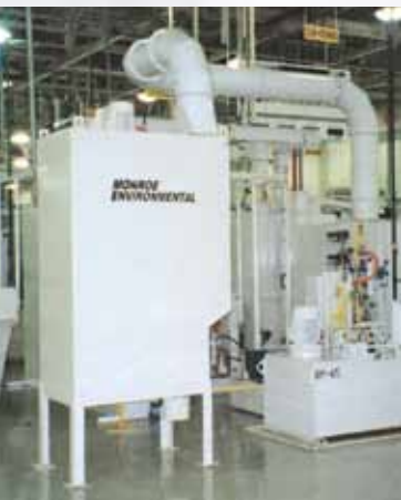
1,500 CFM Spiral Tube Mist Collector for precision machining operation
