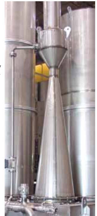
High pressure drop 80 in. W.C. fixed throat Venturi
