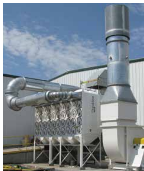
DFO on Corn Husking & Sorting 28,500 cfm (48,412 m 3 /h)
