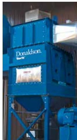
VH on Blasting 14,000 cfm (23,781 m 3 /h)
