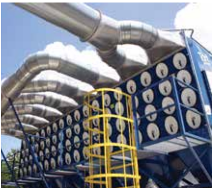
DFO on Sawdust 57,500 cfm (97,692 m 3 /h)
