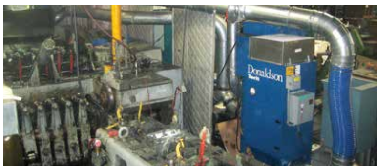
WSO on Cold Forming 1,200 cfm (2,038 m 3 /h)
